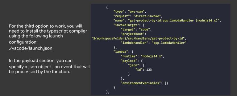
The result of running any of the options is the same - the application is launched locally in debug mode. The plugin uses the same "sam" build and "sam" local invoke commands, just with a different build directory.
